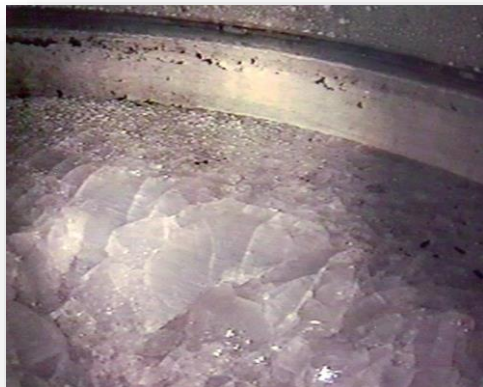
(left) Solid “Frozen” and (right) Liquid “Molten” 2\text{LiF}\text{-BeF}_2 salt
